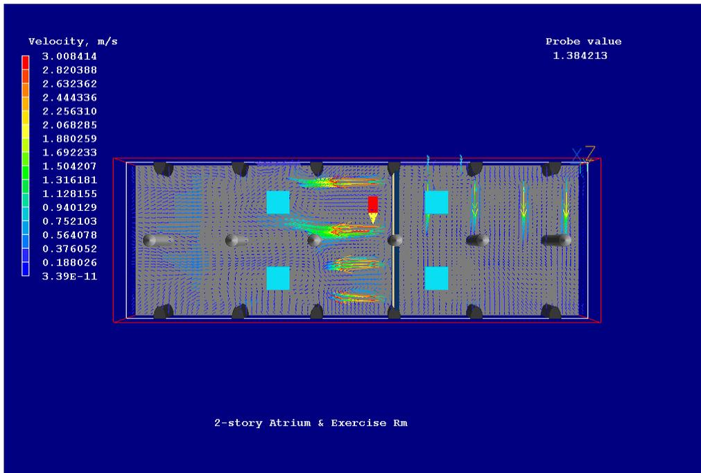
Figure 3.1-d Phoenics Velocity Z Slice 1
