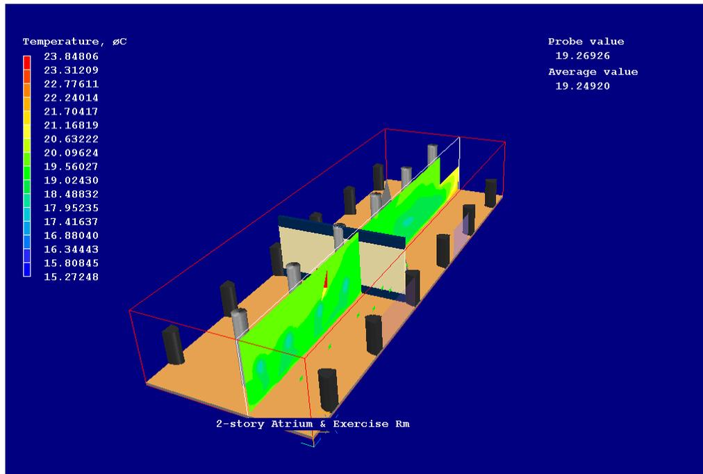
Figure 3.1-k Phoenics Temperature Y Slice 2
